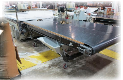
Waste hopper on side of conveyer band
