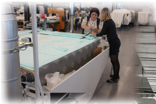
Waste hopper on end of conveyer band
