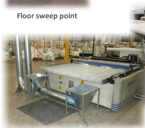
Double waste hopper on end of conveyer band
